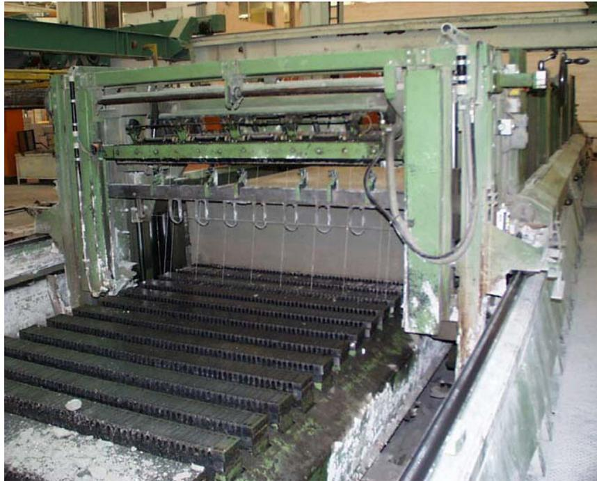
*Figure 2.14: Cutting AAC mass after the forms are stripped (Tanner 2003)*
