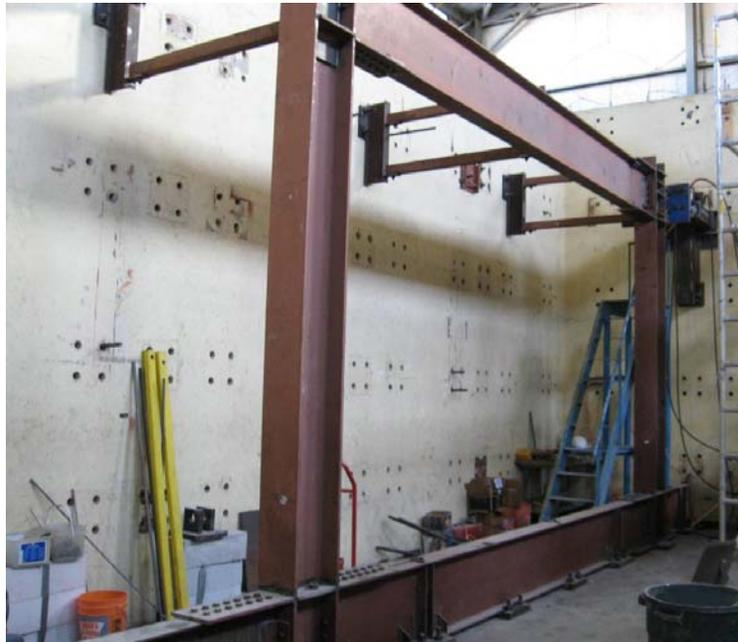
*Figure 4.7: Bare steel moment frame before test*
