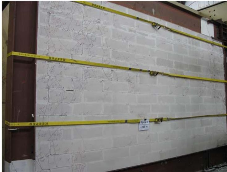
*Figure 4.12: AAC-infilled frame after testing*
