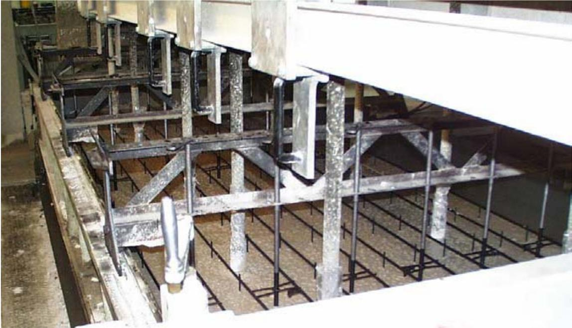
*Figure 2.13: AAC slurry in molds during the rising process (Tanner 2003)*
